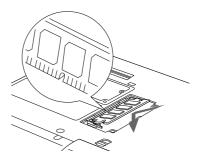
Figure 4-10 Installing a Memory Upgrade Module
